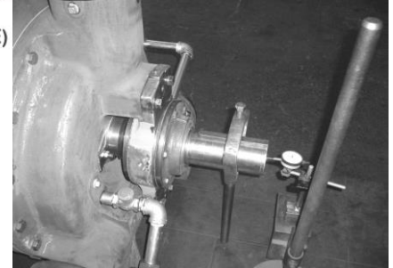
Fig. 30A. Rotor end travel measurement
