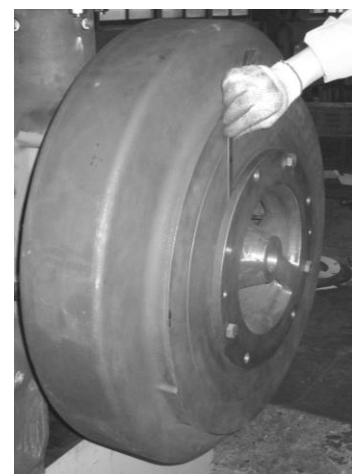
Fig. 37. Measure the gap by feeler gauge
